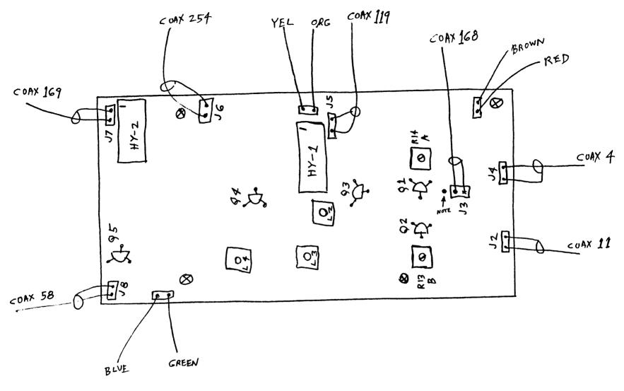
NOTES: 1. GROUND PIN OF J3 IS NOT USED. DNLY THE CENTER CONDUCTOR OF COAX 168 IS PLUGGED IN. PREVENTS GROUND LOOP HUM IN RECEIVER.
